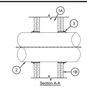
SYSTEM NO. W-L-1001 F RATINGS - 1, 2, 3 AND 4 HR (SEE ITEMS 2 AND 3) T RATINGS - 0, 1, 2, 3, AND 4 HR (SEE ITEM 3) L RATING AT AMBIENT - LESS THAN 1 CFM/SQ FT L RATING AT 400 F - LESS THAN 1 CFM/SQ FT
